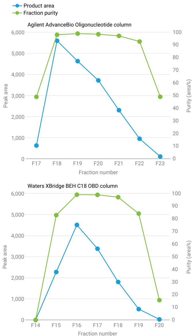
Figure 5. Fraction analysis details using method 2, showing peak area and %peak area for individual fractions.
